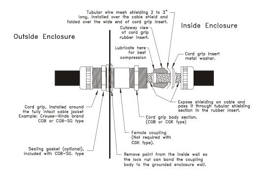
Figure 2: Through Wall Shield Grommet
